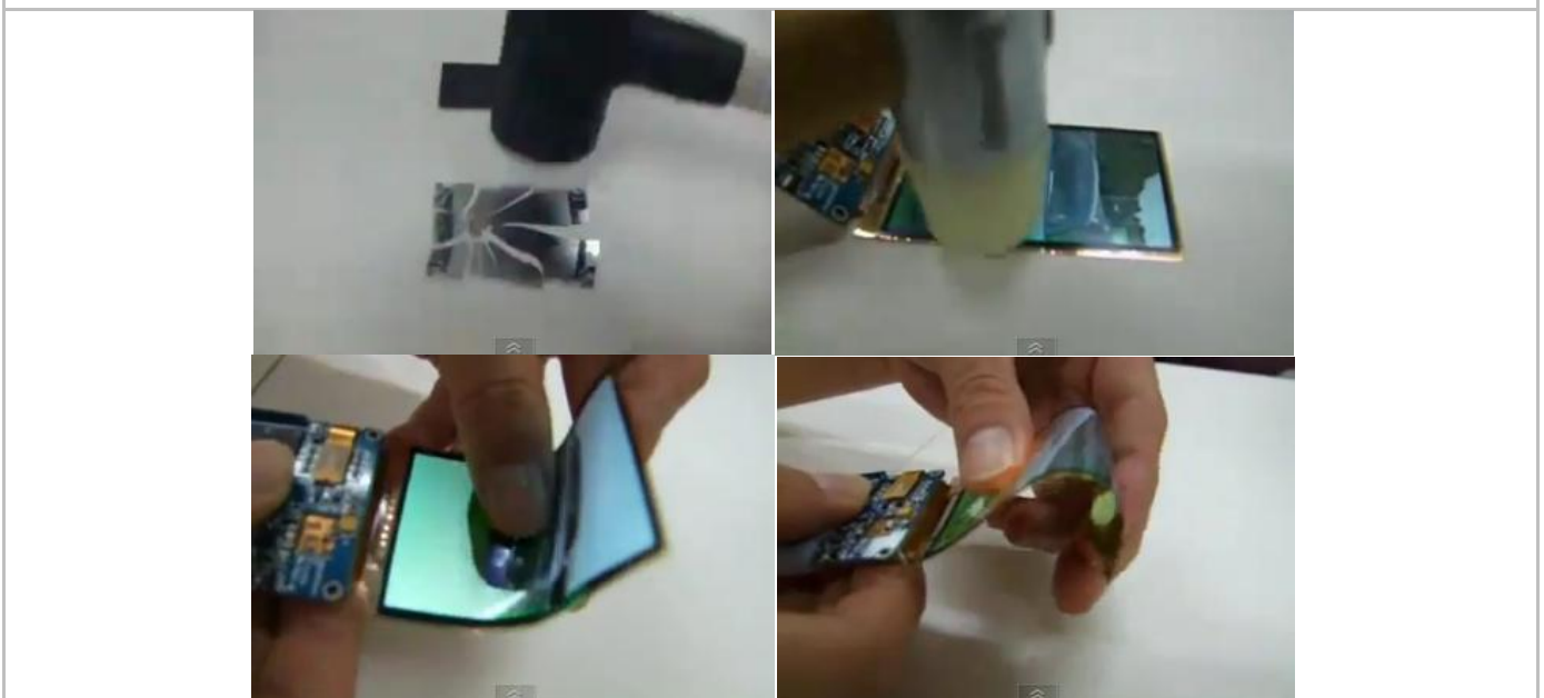
Exhibit 20. SEC's flexible display hammer test (Top left is a general display)
